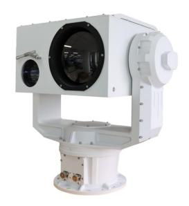
tracking, identification and tracking of targets, and the operating distance can reach more than 20km. The optical platform camera system can be fixedly erected or used in vehicles. It is adopts military quality design, and the overall shell is made of super cast aluminum material, and the protection level reaches IP66/IP67, which effectively ensures the long-term stable operation of the equipment in the harsh field.
